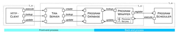
Figure 2: Component diagram of TIRA. Towards the left, the front-end process dealing with the user-interaction is illustrated. To the right, the back-end program execution process is shown. Requests are illustrated by arrows and imply a response from the requested component.
