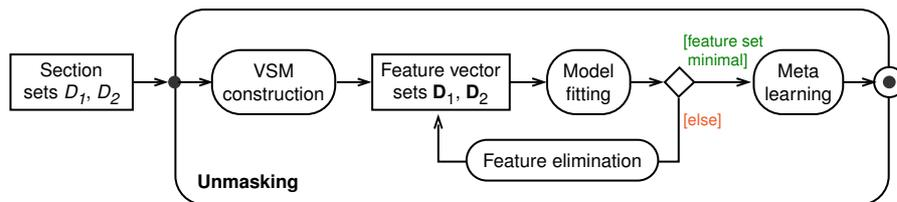
**Figure 2** Given are two sets of sections  $D_1$  and  $D_2$ , allegedly written by a single author. Unmasking measures the separability of  $D_1$  versus  $D_2$  when the style model is successively impaired.
