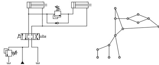
Fig. 9: Circuit with sequentially coupled axes.
