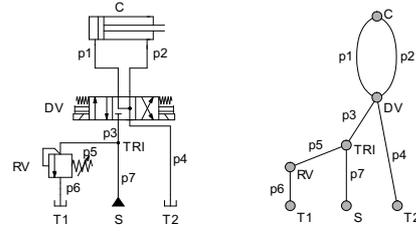
Fig. 5: Sample circuit with its related graph.
