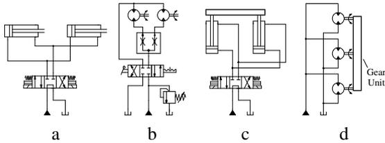
Fig. 3: Hydraulic axes with multiple actuators.
