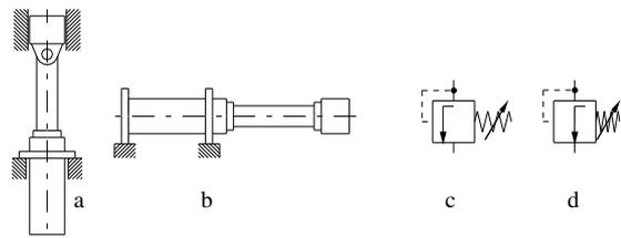
Fig. 2: Examples for arrangement structure (a, b) and switching state structure (c, d).
