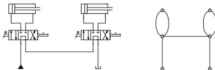
Fig. 8: Circuit with axes coupled in series.
