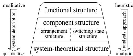
Fig. 1: Structural levels of hydraulic systems.
