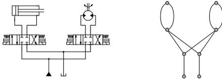
Fig. 7: Circuit with axes coupled in parallel.
